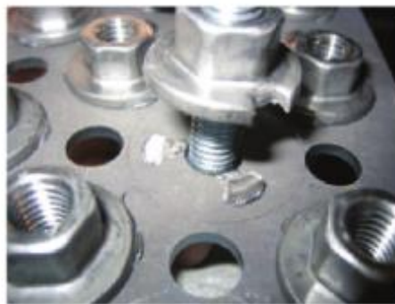
Fig. 4—Here's what can happen during destructive testing of weldments where the fastener and base material have significantly different tensile strengths.
