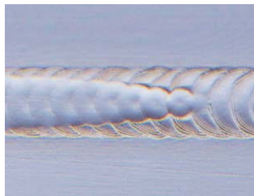
Figure E Fadeout capability on seam welds, to prevent last pulse cracking and ensure completion of smooth seam.
