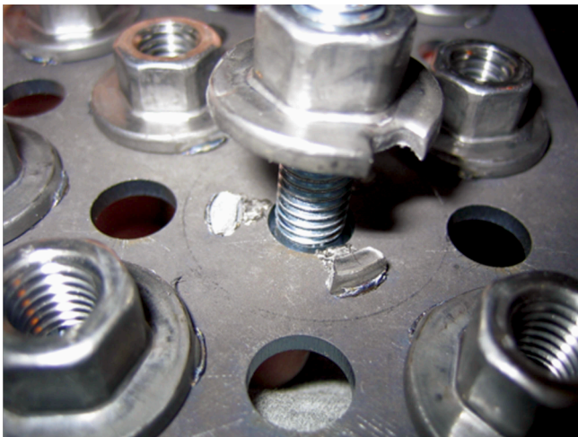
Fig. 2 — A M8 nut welded to 2-mm boron.
